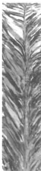
Figure 3.9. Macrostructure in an ingot.
