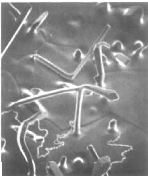
Figure 6.5. Whiskers grown at 1150°C on surface of an iron-aluminium alloy, imaged in an early scanning electron microscope \times 250 (Gardner and Cahn 1966).
