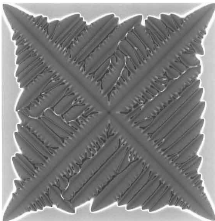
Figure 9.3. Computer simulation of dendrites growing into a Ni–Cu alloy with 41 at.% of Cu. The tints show local composition (courtesy W.J. Boettinger and J.A. Warren).
