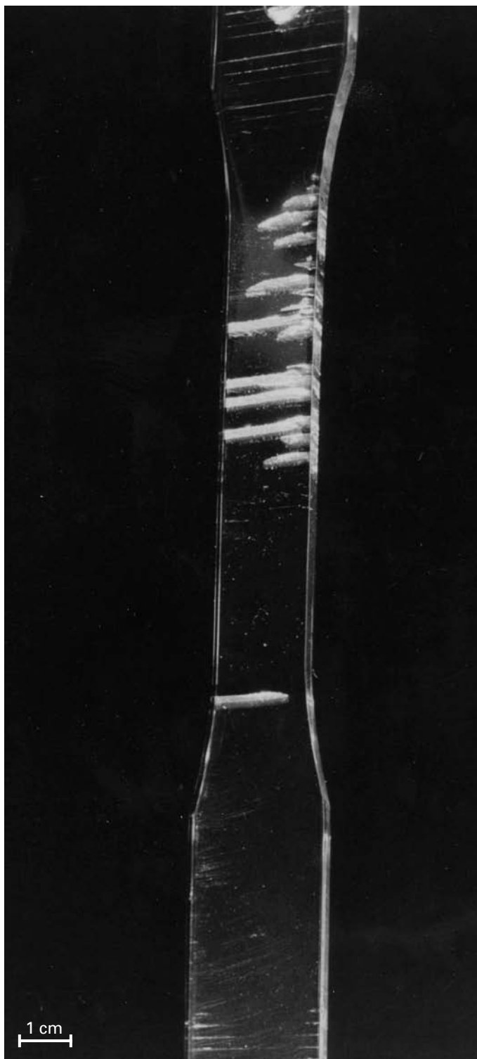
Fig. 8.43 A series of crazes produced in a tensile specimen of polycarbonate. (Used with permission from R. P. Kambour, Polymer , 4 (1963) 143.)
