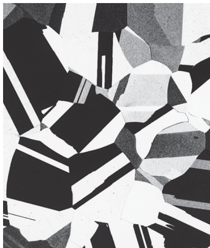
580°C再结晶完成后，700°C保温10min
