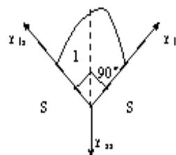
10、解: (1)  $\gamma_{gs} = \gamma_{gl} \cos 70.52^\circ + \gamma_{ls}$
