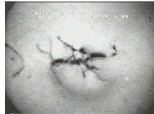
Moving dislocations in molybdenum
