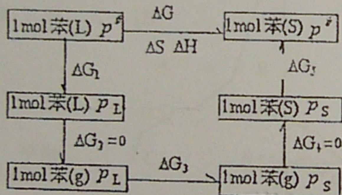
$$\Delta G = \Delta G_1 + \Delta G_2 + \Delta G_3 + \Delta G_4 + \Delta G_5 = \Delta G_3 = nRT \ln \frac{P_s}{P_l} = 1 \times 8.314 \times 268 \times \ln \frac{17.1}{19.8} = -326.65 \text{ J}$$
