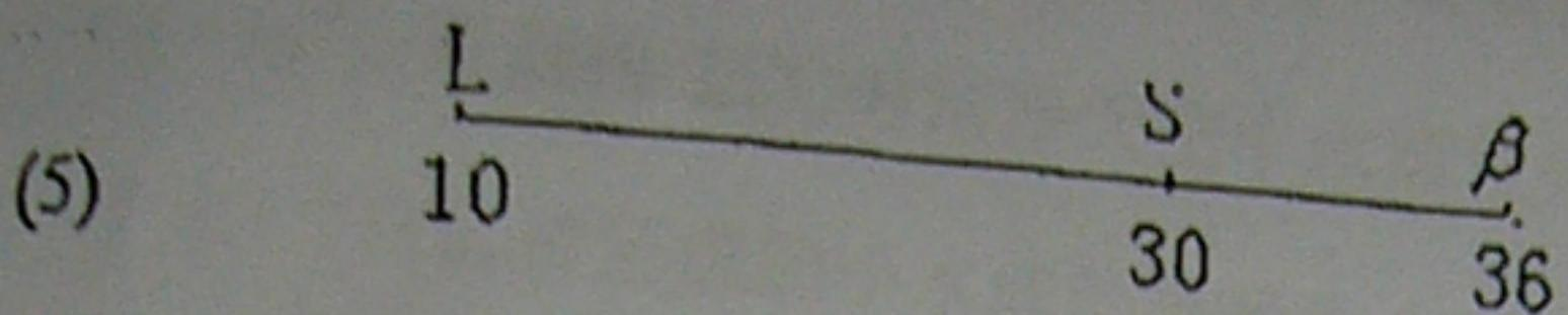
$$\frac{m_\beta}{m} = \frac{30 - 10}{36 - 10} \quad m_\beta = \frac{30 - 10}{36 - 10} m = \frac{20}{26} \times 1 \text{ kg} = 0.769 \text{ kg}$$
