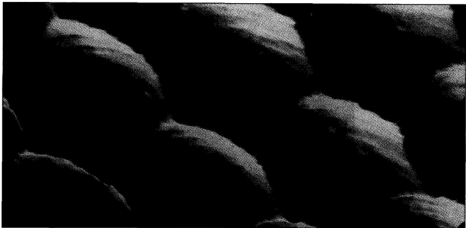
Figure 4.37 STM image of the surface of platinum showing outstanding atomic resolution. (IBM Research, Almaden Research Center.)
