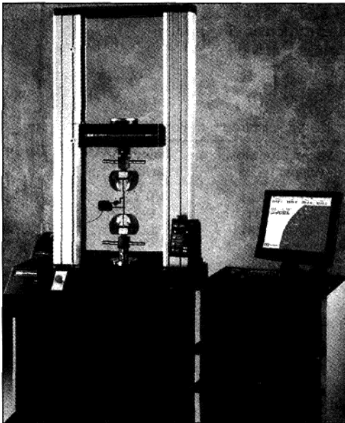
Figure 6.16 Modern tensile testing machine. The force (load) on the specimen is measured by the load cell while the strain is measured by the clip-on extensometer. The data is collected and analyzed by computer-controlled software. (Courtesy of the Instron® Corporation.)
