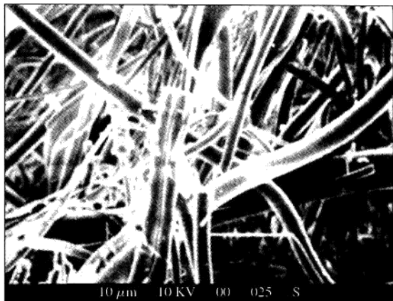
Figure 11.39 Microstructure of LI900 high-temperature reusable-surface insulation (ceramic tile material used for space shuttle); structure consists of 99.7% pure silica fibers. (Magnification 1200 \times .) (Courtesy of Lockheed Martin Missiles and Space Co.)
