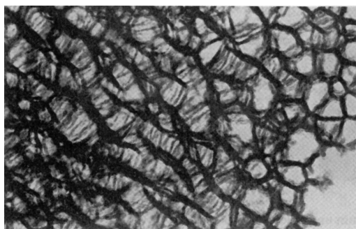
Figure W11.9. Transmission electron micrograph of porous Si in which the Si columns are about 10 nm in diameter and the pore spaces are about 50 nm wide. (Reprinted with permission of A. G. Cullis. From R. T. Collins et al., Phys. Today , Jan. 1997, p. 26.)
